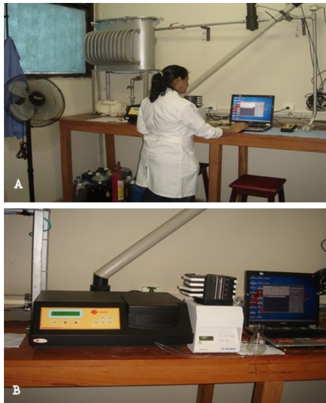
Fig. 1. Pilot unit for simulating insulating oil degradation (A) and Flow Injection Analysis (FIA) coupled to a UV-VIS spectrophotometer (B).
